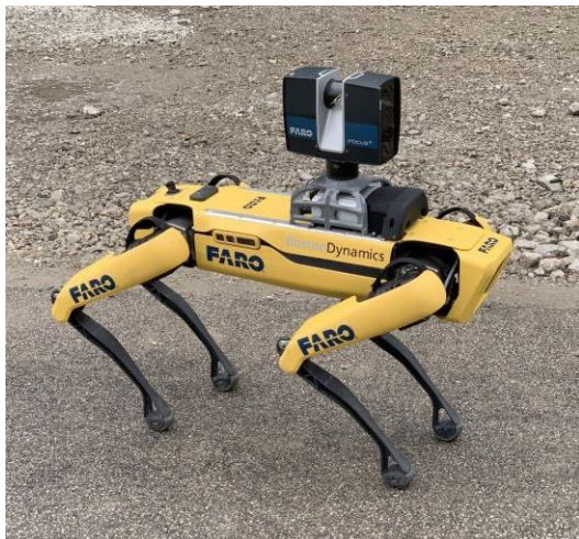
Fig. 14. The integration of FARO Focus scanner and Spot robot dog [81].
