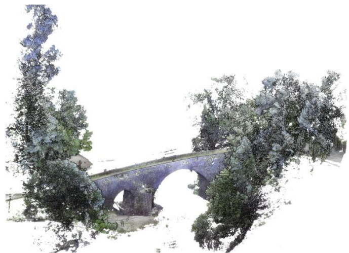
Fig. 3. Acquired point cloud with vegetation (north side).
