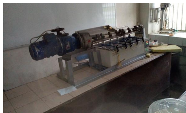
Figure 1: A locally-fabricated fermentor used for the liquefaction
