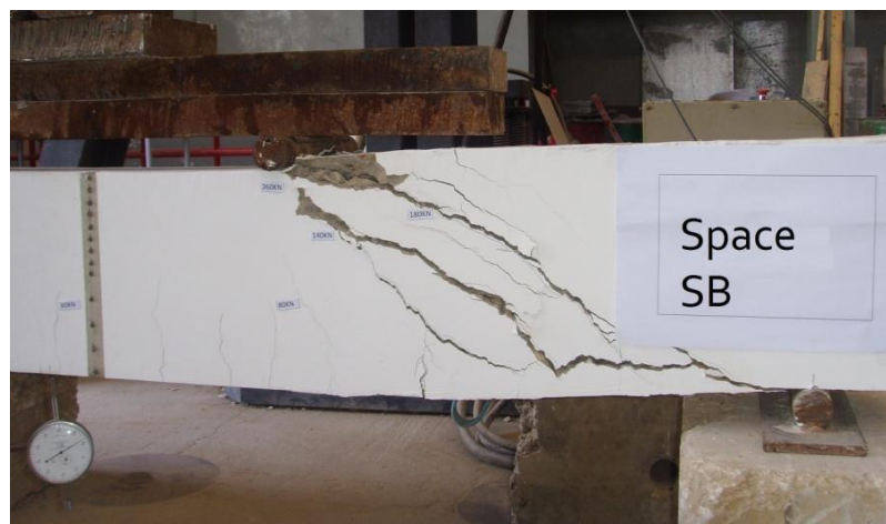
Fig. 7: Typical shear failure.
