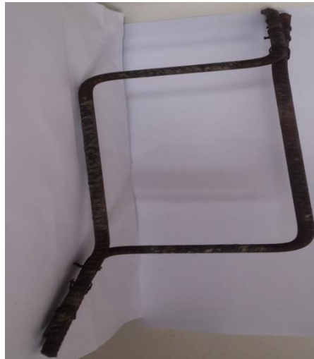
Fig. 3: Assembled space swimmer bars loop.
